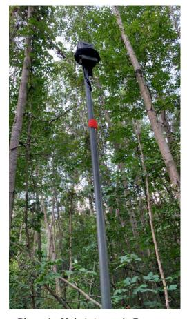
Photo 1: Unit 1 Acoustic Detector
